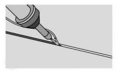
Using specialist equipment, the two pieces are joined or welded together in this case the weld rod is heated and fed into the created joint with a hot air welder.
