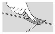
The weld is then trimmed, and excess weld material is removed to give the finished floor.
